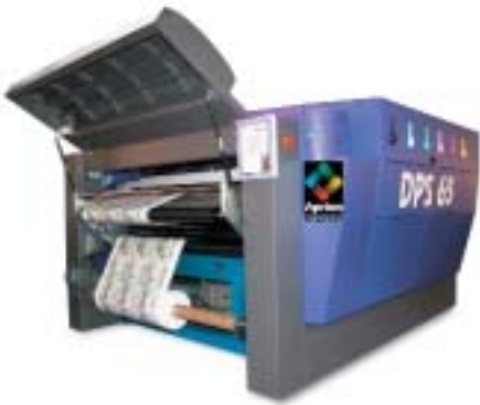
Industrial inkjet press for home furnishing applications - Aprion DPS65
