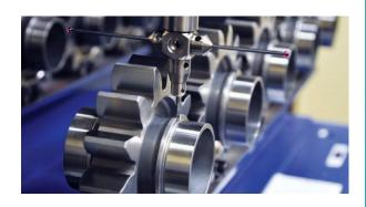
BMT are also able to load CAD models provided by engineering into QUINDOS. Now they can more easily visualise and create their inspection routines in an intuitive CAD based environment.
