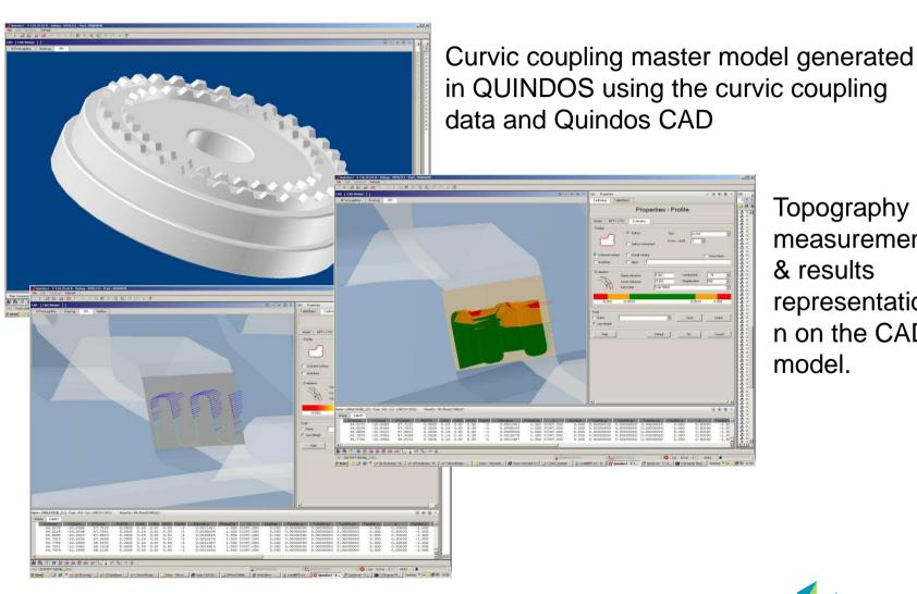
Topography measurement & results representatio n on the CAD model.
