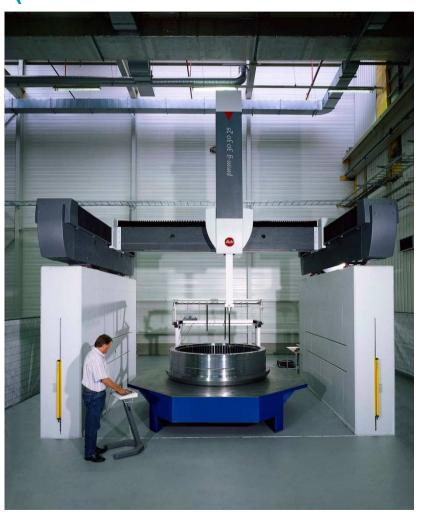
Gantry Type CMM for Gear Diameter up to 3700 mm
