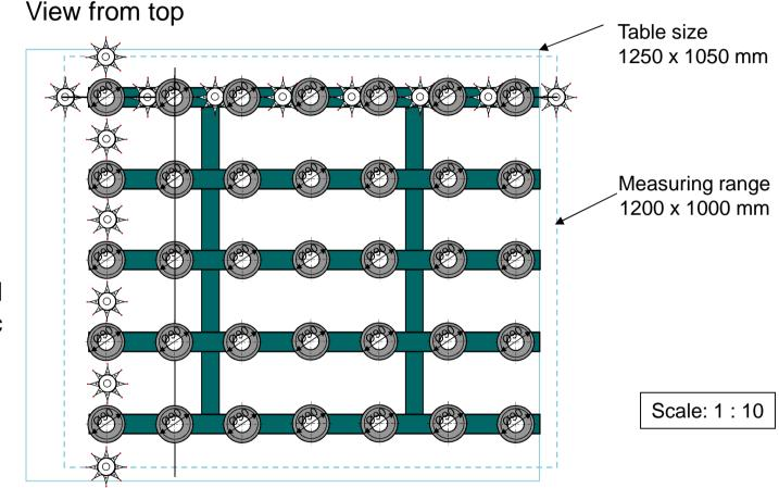
Measuring range required in Y (for gear dia. 90 mm, with 5mm clearance for moving):  $50 + 5 + (5 \times 90) + 4 \times (5 + 100 + 5) + 50 + 7 = 1000$  mm
