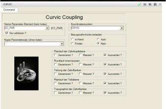
The Quindos Curvic Coupling option can be used to calibrate Curvic Coupling gauges used to check Curvic Coupling parts. The actual geometry is compared to the theoretical geometry in order to determine the pairing characteristics of the Curvic Coupling.
