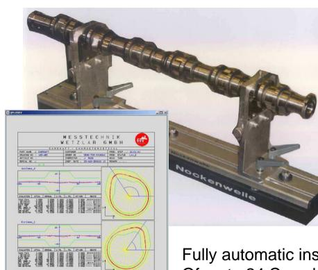
Fully automatic inspection Of up to 24 Camshafts On 1 fixture!
