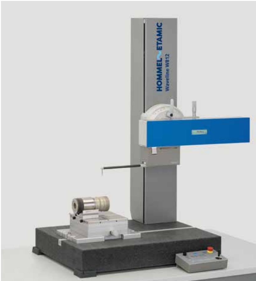
Waveline W812 Digiscan with 500 mm measuring column and 120 mm traverse unit
