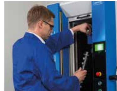
Simple operation of the measuring machine thanks to fast tailstock adjustment
