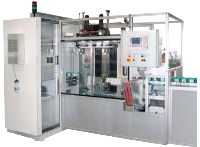
Automated Opticline for measuring engine valves; integrated in a production line
